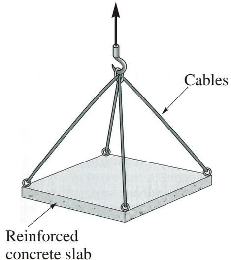
Fig. 2 A reinforced concrete slab is lifted by 4 tensile cables
