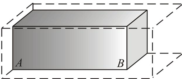
Fig. 18 Block of material subjected to an increase in temperature
