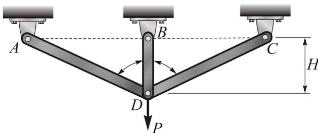
Fig. 9 A vertical load  $P$  is supported by the truss  $ABCD$  which are pinned connected and
