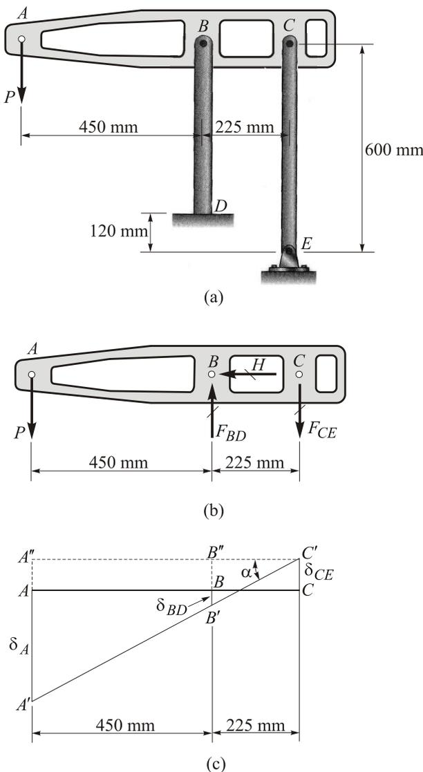
Fig. 20 Horizontal absolutely rigid beam  $ABC$  supported by 2 vertical bars
