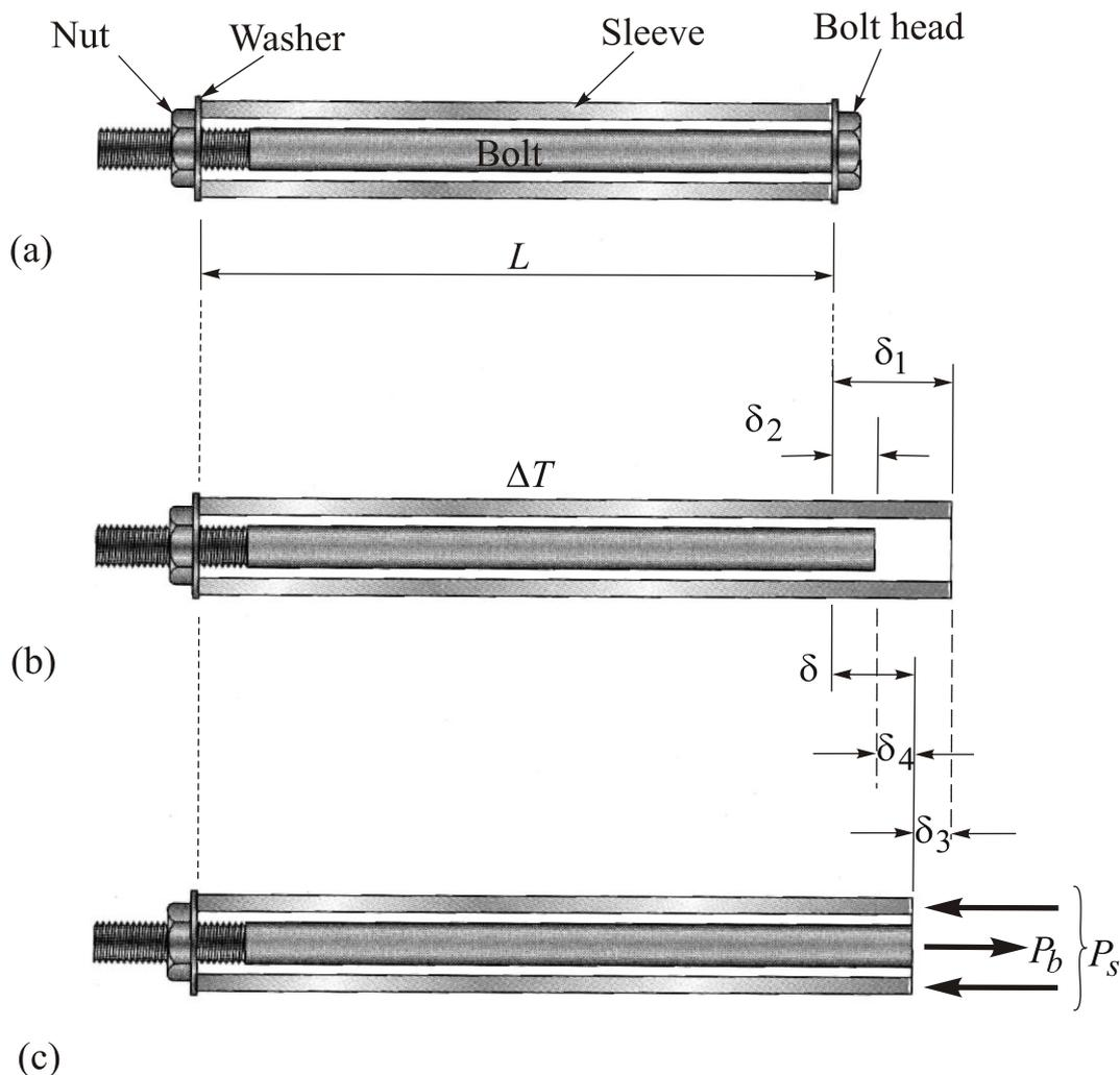
Fig. 28 Sleeve and bolt assembly with uniform temperature increase  $\Delta T$
