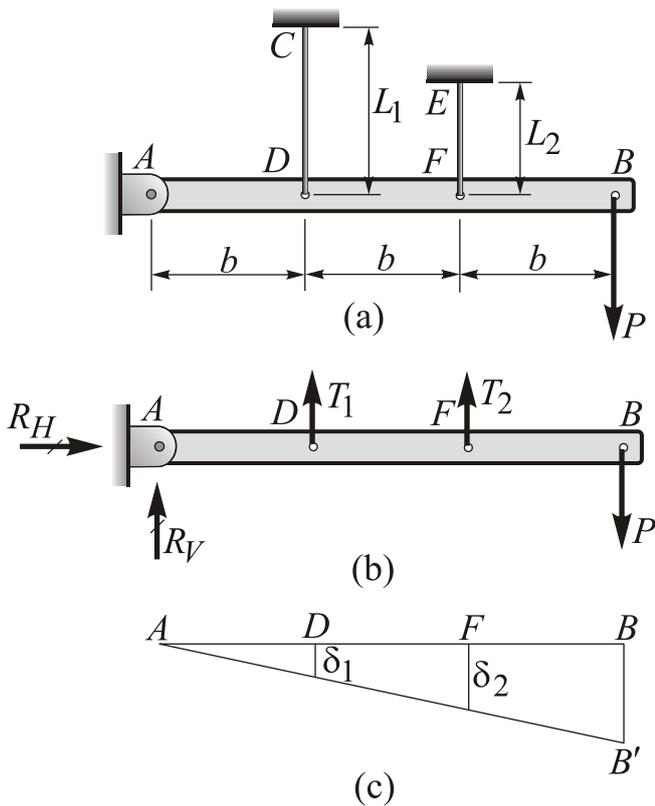
Fig. 26 Analysis of a statically indeterminate structure
