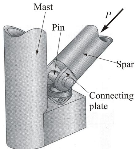
Fig. 13 An aluminum bar  $AB$  is attached to a support by a pin and is tensile by a  $P$  force
