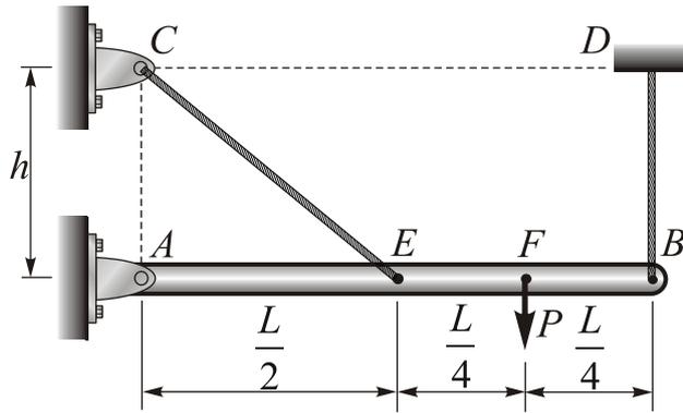
Fig. 15 A rigid bar  $AB$  is supported by two cables  $CE$  and  $BD$  which are tensile under  $P$  loading
