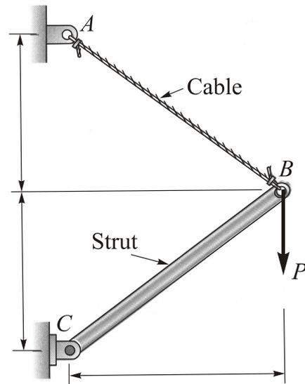
Fig. 8 A cable and strut assembly  $ABC$  supports a vertical load  $P$ . The cable and strut are in tension-compression.
