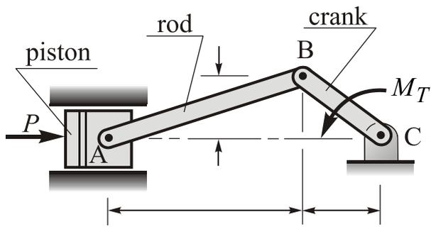
Fig. 5 The piston in an engine is attached to a connecting rod  $AB$ , which intern is connected to a crank arm  $BC$ . Both elements are compressed or tensile
