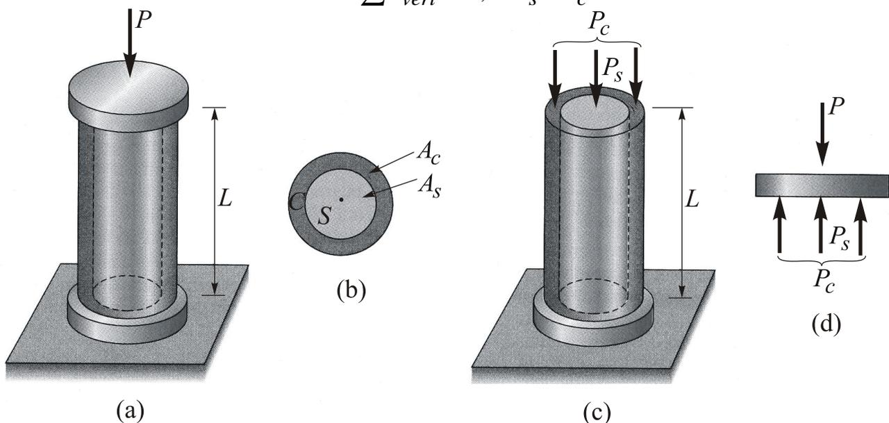
Fig. 25 Analysis of a statically indeterminate structure
