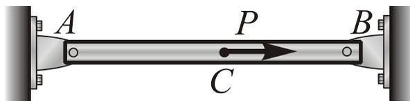
Fig. 21 The picture of statically indeterminate rod loaded by concentrated force at point  $C$ .  $A$  and  $B$  – immobile hinged supports
