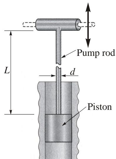
Fig. 4 A pump moves a piston up and down in a deep water well. Pump rod is periodically tensile or compressed
