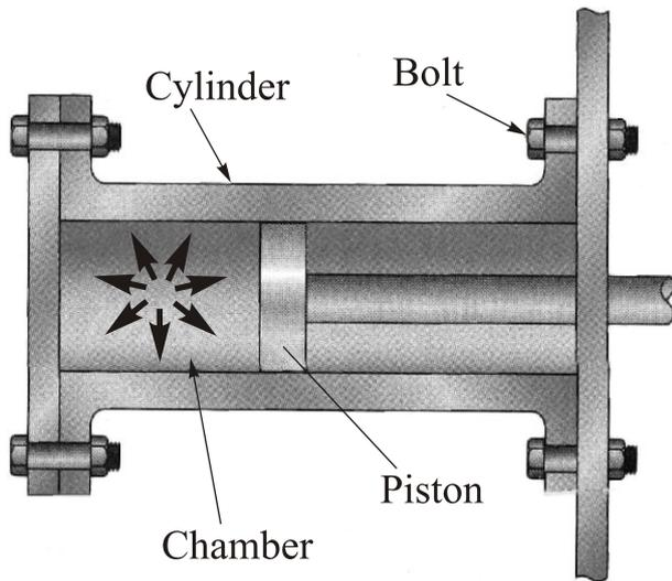
Fig. 7 Cylinder with piston and clamping tensile bolts
