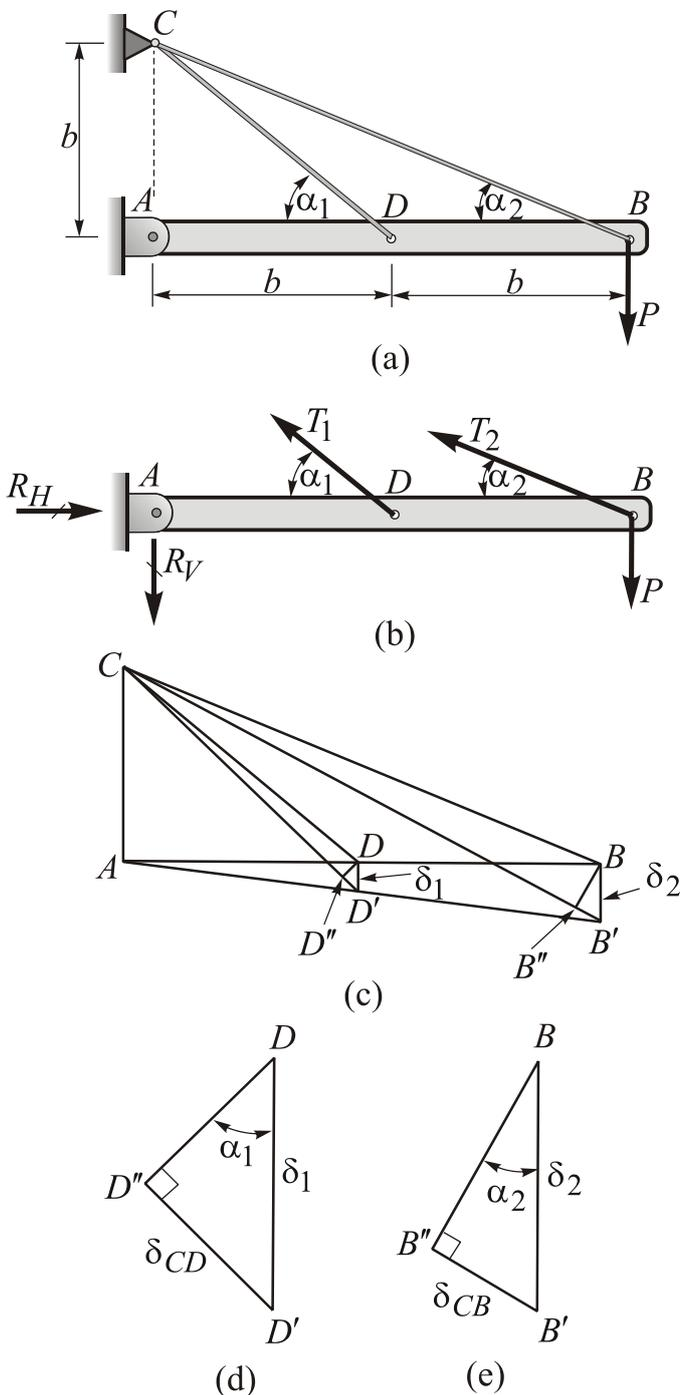
Fig. 27 Analysis of a statically indeterminate structure
