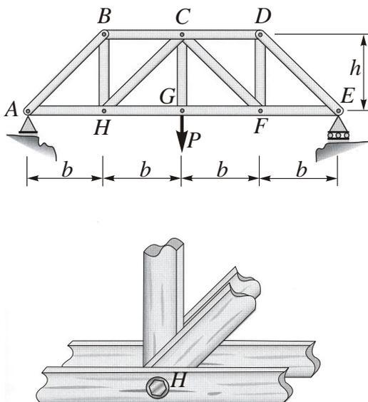
Fig. 3 The truss  $ABCDEFGH$  is part of a wood bridge. The truss members are hinged
