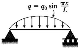
$$v = -\frac{q_0 L^4}{\pi^4 EI} \sin \frac{\pi x}{L} \quad v' = -\frac{q_0 L^3}{\pi^3 EI} \cos \frac{\pi x}{L}$$
