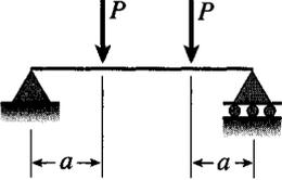
$$v = -\frac{Px}{6EI}(3aL - 3a^2 - x^2) \quad v' = -\frac{P}{2EI}(aL - a^2 - x^2) \quad (0 \leq x \leq a)$$
