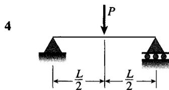
$$v = -\frac{Px}{48EI}(3L^2 - 4x^2) \quad v' = -\frac{P}{16EI}(L^2 - 4x^2) \quad \left(0 \leq x \leq \frac{L}{2}\right)$$
